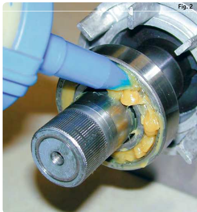
Greasing a deep groove ball bearing mounted on a rotor shaft
